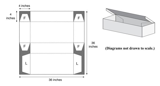
The shaded areas are cut away and the rest is folded along the dashed lines. The sides are folded up and stuck together using the four flaps marked F.
